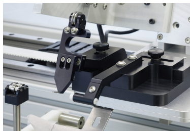
Quick change tooling base with two pin guide tooling. Also shown is the roller-style mandrel damper.
